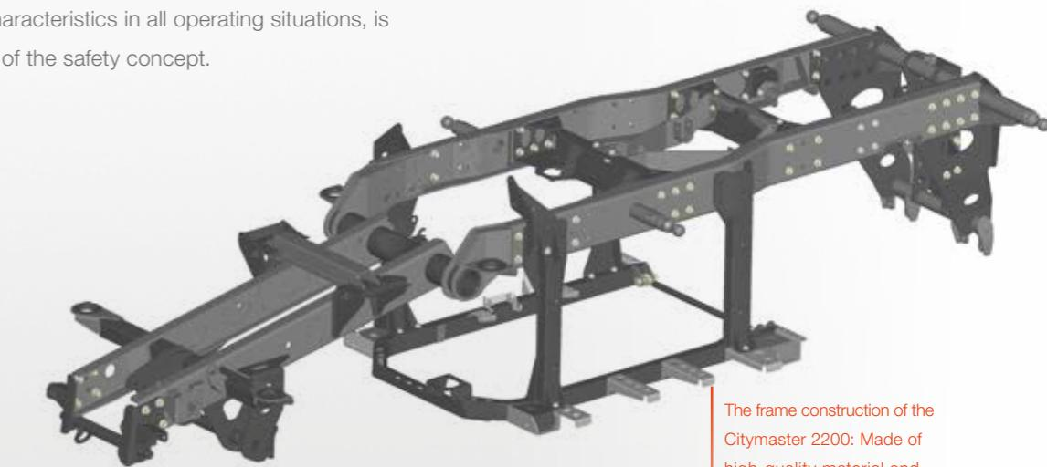
The frame construction of the Citymaster 2200: Made of high-quality material and manufactured in Germany, robust and non-deforming – a safe basis.
